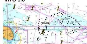
Within the windfarm a seaweed farm has been established. The site is marked by 4 yellow buoys. The lines and buoys are in the surface in the seaweed farm at Danish Kriegers Flak and navigation within the marked area should be avoided.
